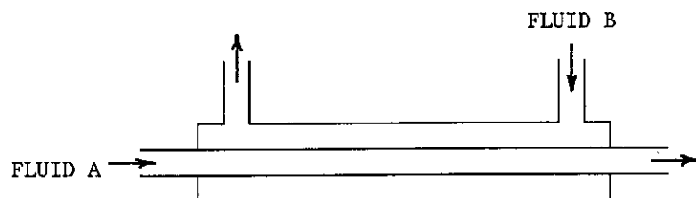
FIGURE (43-1) HEAT EXCHANGER FOR PROBLEM (43-1)
